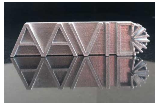
Figure 1 – Additive Manufacturing Prototype of Aavid, Thermal Division of Boyd Logo
