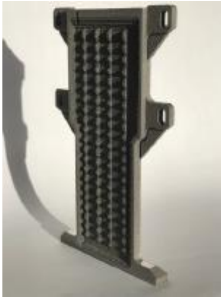
Figure 6 - Future Integrated AM Heat Pipe Vapor Chamber Proof-of-Concept
