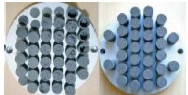
Figure 3 - AM Laser Parameter Trial and Optimized Parameter Build Plates Comparison
